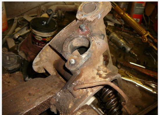
Oh no, broken studs.
