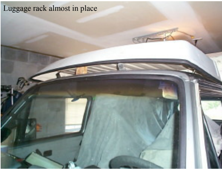
The poptop is bolted on.
