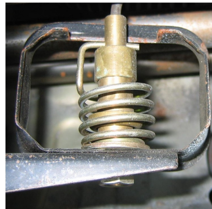
Photo 4 - Modified Bracket - Note material cut away at top of bracket to allow spring to clear bracket when thermostat expands. (Photo by Stan Wohlfarth)
