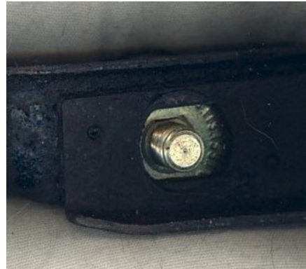
Photo 3 - Old Bracket with New Thermostat Securing the bottom of the new thermostat to the old bracket can be done with a washer/nut, but alignment in the hole is sloppy.
